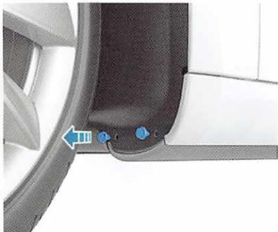
4. Open the front-most rocker panel bolt access cover, and then remove the bolt and washer.
