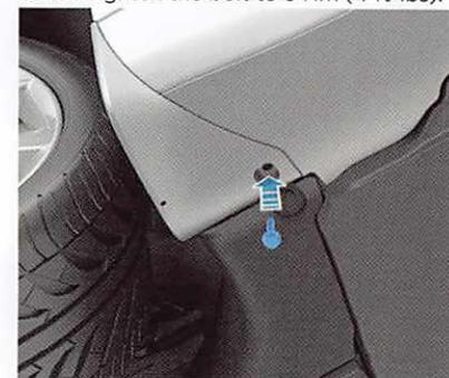
10. Perform this procedure again on the right side of the vehicle to install the right mud flap or splash guard.
