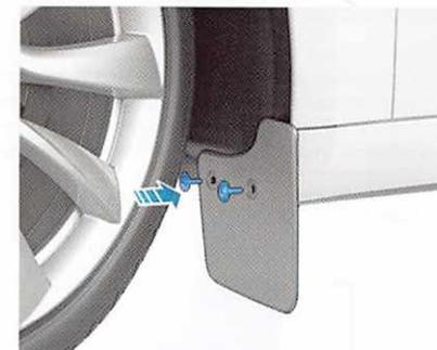
9. Install the bolt that secures the bottom of the mud flap to the lower rocker panel cover. Tighten the bolt to 5 Nm (4 ft-lbs).
