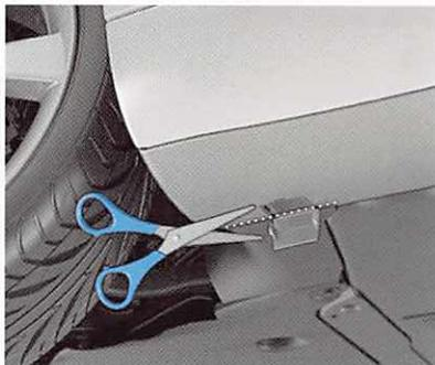
6. While carefully pulling the lower portion of the front wheel arch liner away from the wheel well, install the U-nuts (x2) over the holes in the rocker panel. Make sure the holes are aligned.
