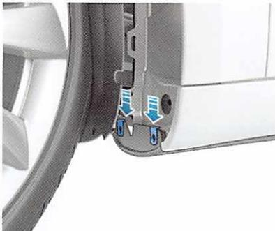
7. **IF INSTALLING SPLASH GUARDS:** Remove the adhesive backing from the splash guard, and then align the splash guard with the mud flap so that the holes are aligned. Once aligned, apply pressure along the mud flap to ensure it is adhered to the splash guard.
