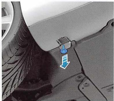
5. Carefully use scissors to remove the open access cover from the rocker panel.
