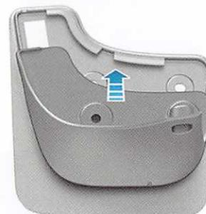
8. Place a washer over the screws (x2), and then install the screws to secure the mud flap/splash guard to the U-nuts in the front wheel arch liner. Tighten the screws to 1.5 Nm (1 ft-lbs).
