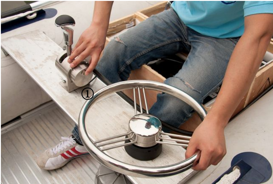
①:press the power switch
